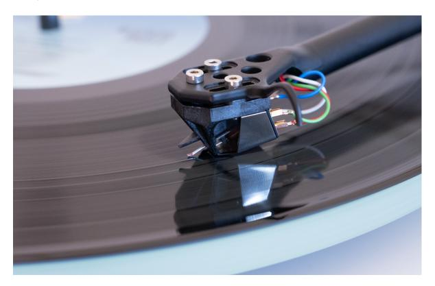
tightening and stripping the threads but Rega says that these are good for more than the 0.4nM provided by their cartridge torque driver, and tell me that they have gone as far as 1.5nM before something gave out. And that something was the hex head of the bolt rather than the cartridge body. Using the relatively short Allen key that Rega supplies pretty well ensures that you can't over tighten the bolts.
